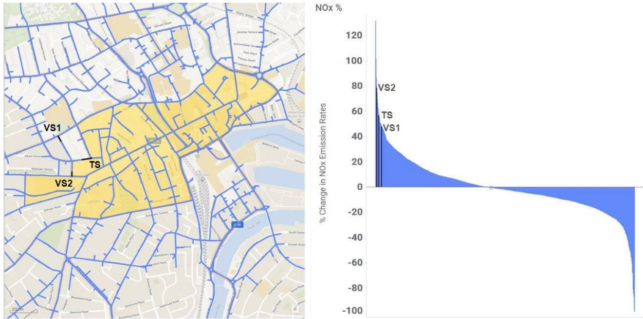
Figure 9. The highlighted sections of Victoria Street (VS1 and VS2) and Thistle Street (TS) see over a 40% increase in NO x emissions. The extent of the LEZ is shown in yellow.
